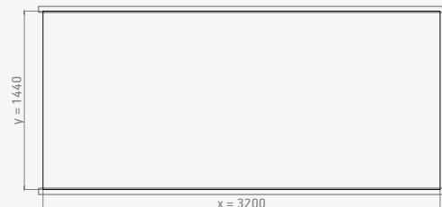
H1. Max. Design wind load: 0.5 kN/m²
