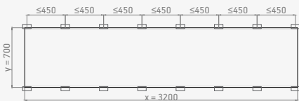
H1. Max. Design wind load: 1 kN/m 2
